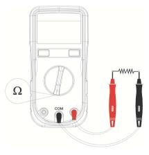
5-1. Apply the red test lead to "V $\Omega$ mA" terminal , the black one to "COM" terminal.
